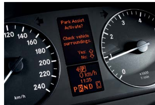
The display in the instrument cluster provides information on the parking manoeuvre
