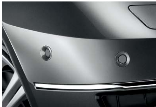
Proximity sensors in the front and rear bumpers monitor the distance to the nearest vehicle or obstacle
